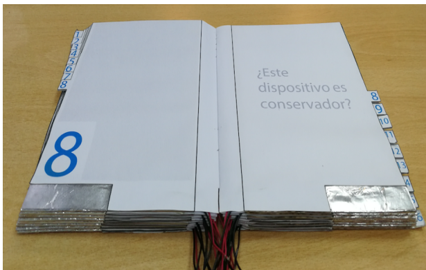
Figure 5: Book used magnets of 1mm thickness.
