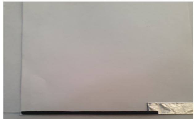
Figure 2: Aluminum foil was added over the conductive paint.
